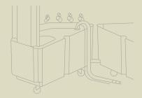
Put the lid plugs on the left and right oval tank openings on the lids.
