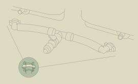
Check the two red locks located at the ends of the drainage valve tubing are in the open position. This is when the red locks are closest to the elbow joint in the tubing.
