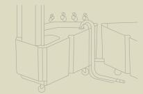
Put the lid plugs on the left and right oval tank openings on the lids.
